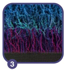
The filament-like structure of the eG Coating allows interdigitation of the PLGA coating, forming a strong bond.
